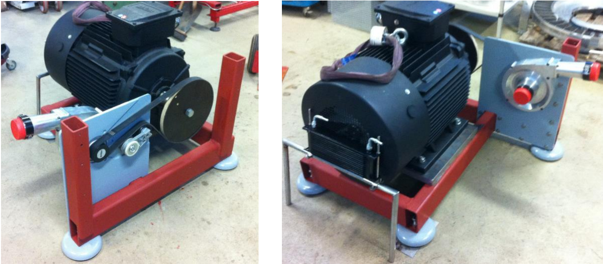
Figure 8: The prototype compressor installed with a standard 50 kW electrical motor, pulley and belt drive
