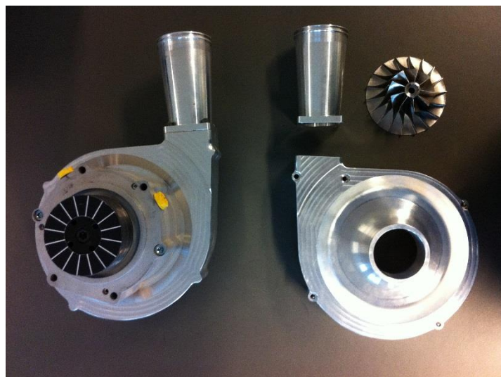
Figure 7: The final compressor prototype compressor including the Rotrex gear (left)
