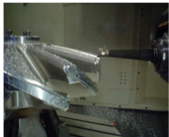
Figure 6 Left: An example of the finite element analysis of a blade in order to minimize the peak stress level. Right: the machining of one of the rotors.
