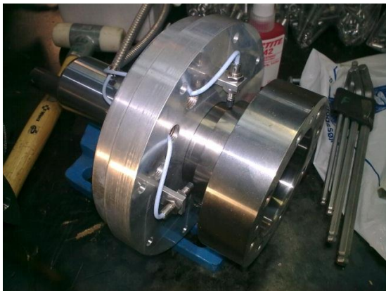
Figure 8 The location of proximity sensors in order to monitor bearing performance.
