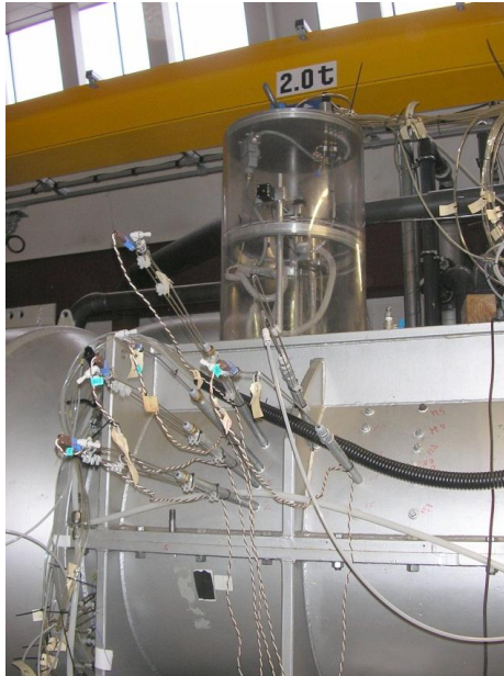
Figure 9 To the left it appears how the pressure and temperature measurements of the compressor performance were made primarily by sensors in the compressor house and partly by a robot on top. To the right it appears how vacuum is maintained by means of a Roots pump and a rotary vane pump.
